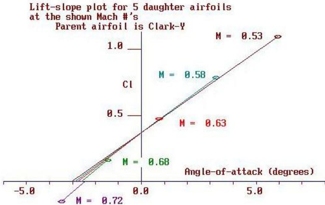
There are 5 different Mach numbers, requiring 5 different “daughter” airfoils. At the high-end of each line is a circle. Use of lift coefficients above this circle will produce shock waves. Hence angles-of-attack which produce higher lift coefficients than those above are forbidden! (The example we analysed for  $M = 0.6$  is not on the above plots).
