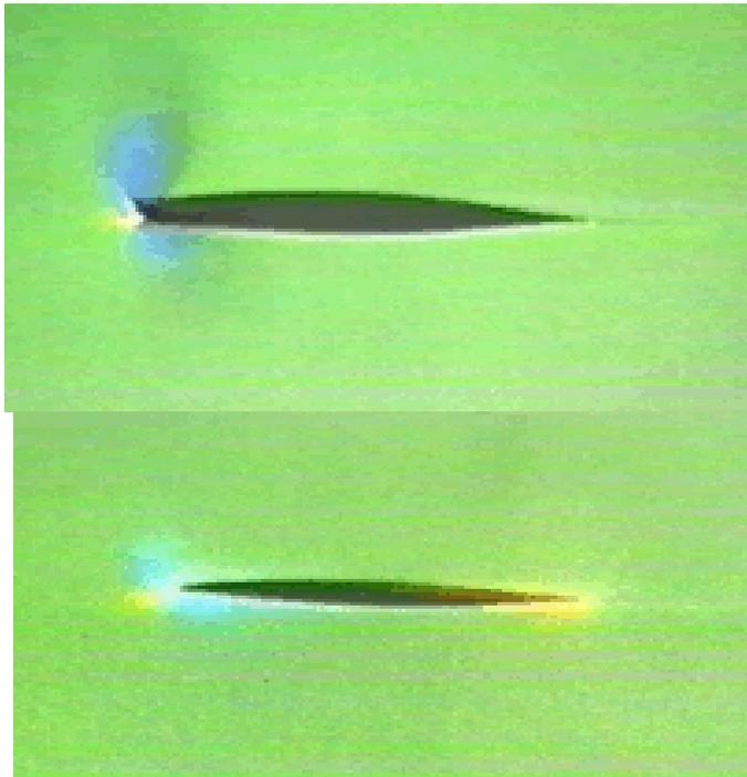
Same airfoils again, this time at higher airspeed with a slight increase in angle of attack. The blue areas of reduced pressure are greater, in proportion to the increased speed of flow over the airfoil
