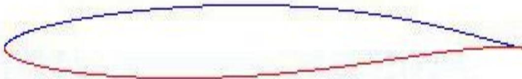
Minimum velocity: increased thickness
