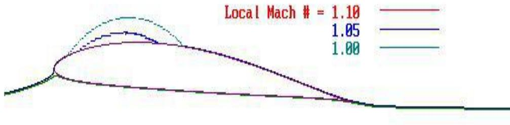
The above plots show the local Mach number, assuming incompressible flow with no shock wave formation. The local speed of sound over the upper surface in both diagrams exceeds the speed of sound at the surface of the airfoil. The local Mach number is reduced by reducing the angle of attack. Regrettably, shock waves DO form so we have a problem!
