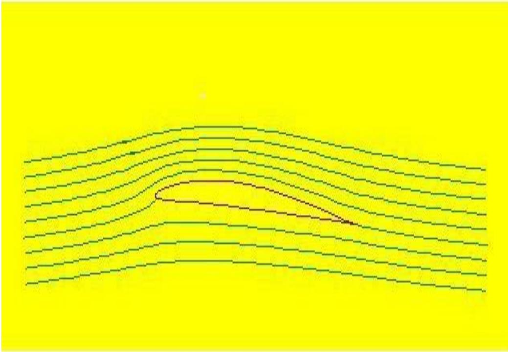
In the plot of streamlines above, the separation of the adjacent streamlines is a guide to the local airspeed and local pressure. On the upper surface, the streamlines are close to each other, indicating increased speed and lower pressure: this surface is called the “suction” side. On the lower surface, the streamlines are further apart, indicating lower local air speed and higher pressure: this surface is called the “pressure” side.
