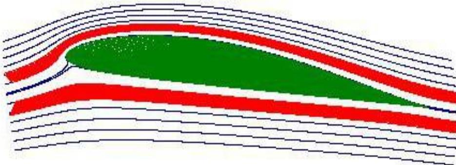
Figure 2: Velocity along streamlines for incompressible flow computed using Joukowski-Jones transform. Observe upper surface velocity increased, lower decreased.
