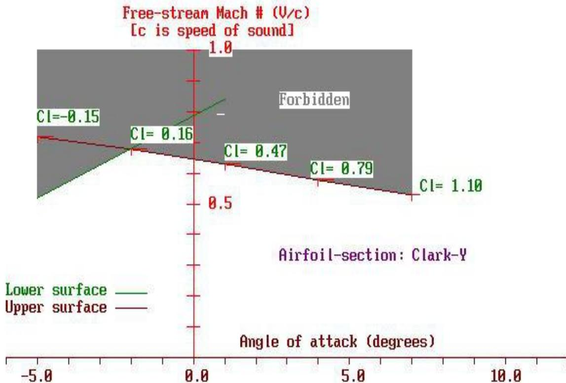
There is a lot on this chart, so look closely. Starting with the axes, we have the abscissa as the angle-of-attack in incompressible flow. The ordinate is the free-stream Mach number. The points for our set of Clark-Y airfoils above are marked in blue, with their corresponding lift coefficients written in next to them.
