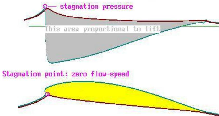
The stream-lines here tell an amazing story. Not only do the streamlines on the upper surface go faster than the free-stream, but the stream-lines on the under-surface go slower than the free-stream (Ref. 1). Not only that, but the streamlines do not part at the leading edge, but rather at a point under and rearward of the leading edge (Figure 2)!
