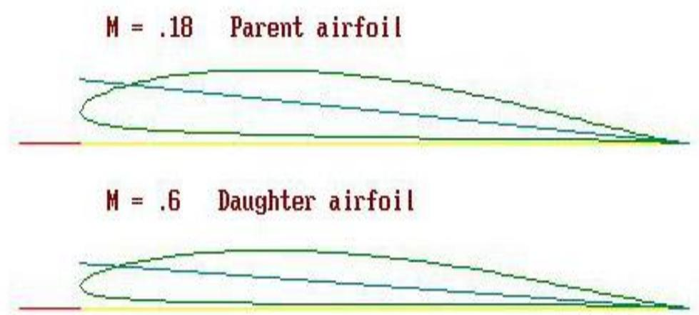
The “parent” airfoil is Clark-Y at Mach .18, due to forward motion of the aircraft.
