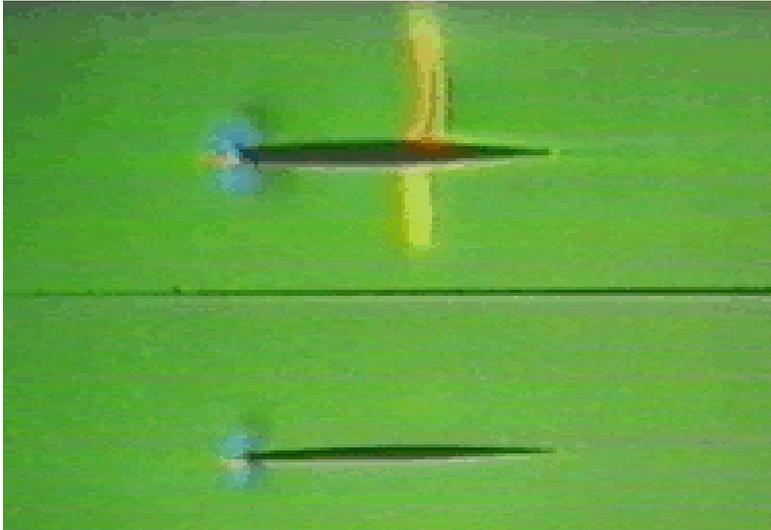
Finally, we return to the thick and thin airfoils, this time at yet higher speeds. Both airfoils are at the same speed of flow. However, the critical Mach number has been exceeded on the thick airfoil, with shocks appearing on both upper and lower surfaces. The local flow speed on the thin section remains below the critical Mach number, so no shock has yet arisen on the surfaces.
