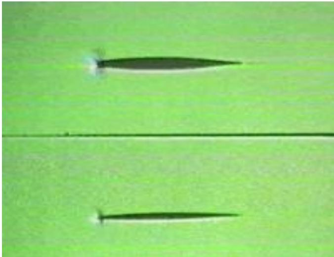
The two images at left show a thick airfoil and a thin airfoil at low speed. The blue area at the leading edge indicates reduced pressure. This is the region of “incompressible” flow.
