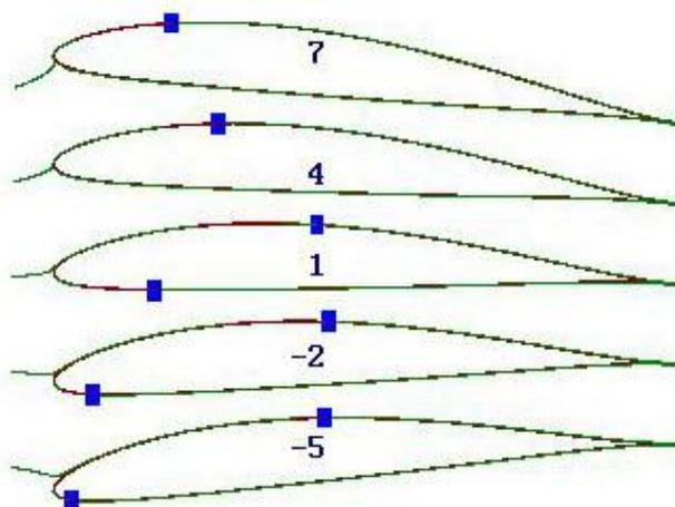
Clark-Y airfoils showing the location of the critical Mach number for various angles-of-attack. Clark-Y is the “parent” airfoil. The calculations are performed as though the air were incompressible.
