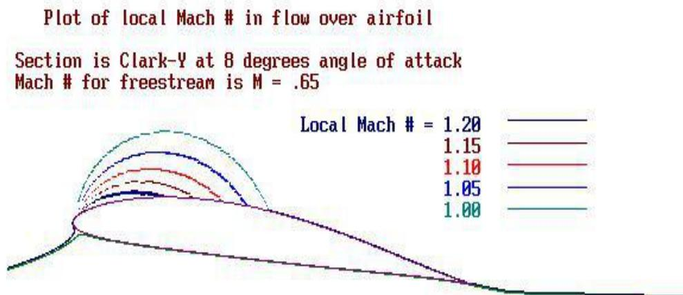
The figure, below, better illustrates the real-world cussedness of transonic flow. As speed is increased, a small region is reached where the speed of flow is supersonic. Instead of then slowing down nicely, there is a sudden change in the behaviour of the air. A shock wave grows out from this point, growing taller with increased intensity as the speed continues to increase. This is the weird behaviour we need to understand.
