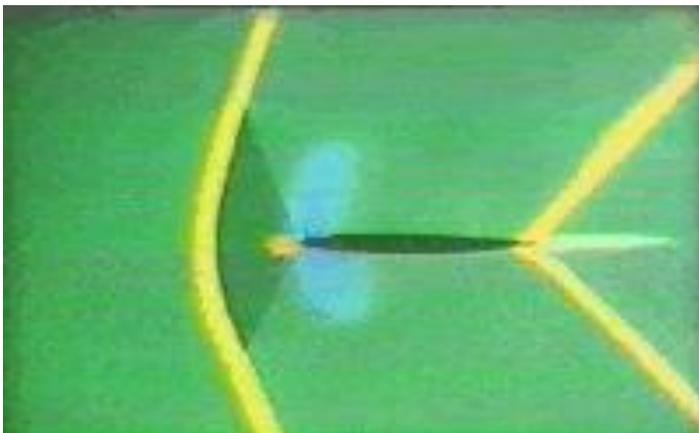
The tunnel speed is now supersonic. A bow wave (detached leading edge shock) has formed, behind which lies a subsonic area (dark green). At the leading edge, the high pressure at the stagnation point remains, as do the low pressure areas (in blue). Behind the leading edge, the flow speed has again increased to supersonic speed leading to further shocks at the trailing edge.
