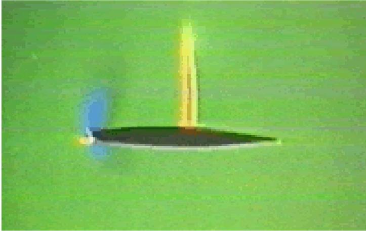
The image at left arises as the speed of flow in the wind tunnel is increased further. This time, the critical Mach number has been exceeded, with a strong shock wave formed on the upper surface.
